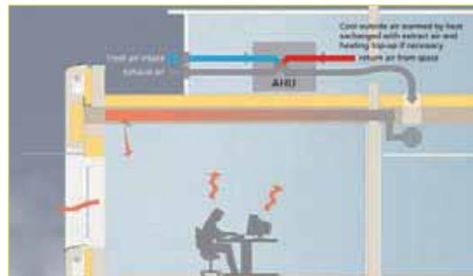
During winter days, cool outside air is warmed by heat exchangers with extract air and heating top-up if necessary (© TermoDeck)
